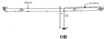
b. Analyse the structure shown by moment distribution method.
